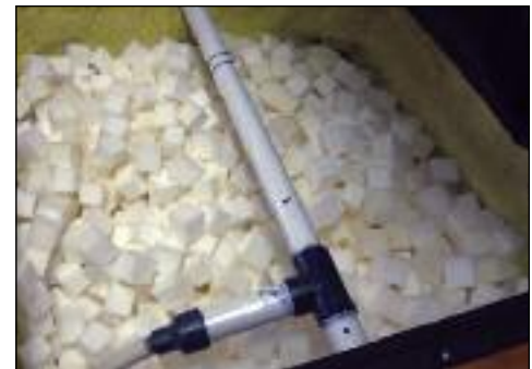
Synthetic media — foam cubes (top view).
